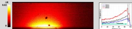
Fig 2. Thermoreflectance 300µm x 100µm map of the facet of NIF LD operated at 1000mA (left). Thermoreflectance signal distributions across the facet at different driving currents (right).
