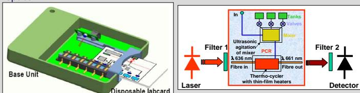
Concept of OPTOLABCARD hand held base unit and a labcard (left) and scheme of the card (right) integrating microfluidical, optoelectrical and microbiological devices
