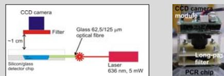
Measurement set-up of the detection unit with CCD camera/filter module: scheme (left) and real picture (right) of the stand
