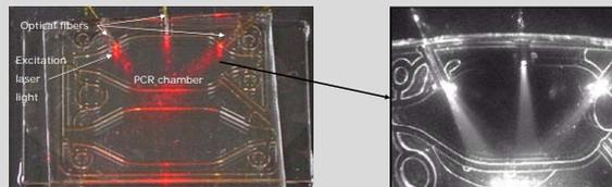
Top views of PCR chip made of glass and SU8, developed by MIC (Technical University of Denmark), on the testing stand (left) and real picture of the sample, containing 250 ng/ml of salmon sperm DNA labelled by TO-PRO 3 fluorochrome, irradiated simultaneously by three optical fibres, the picture captured by CCD camera equipped with 650 nm long-pass filter (adjusted to emission wavelength of TO-PRO 3 fluorochrome)
