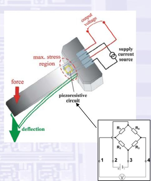
The piezoresistive circuit of ITE sensor contains:
