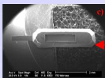
a) Depression for contact pads for protecting the bonding area. b) Tips on the end of the cantilever to make it rough and to improve gripping of an object c) Deep cavity for repeatable positioning and gluing sensor to the gripper.
