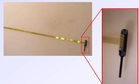
Sensor with elastic lead for easy connections
