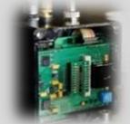
**Vagus Nerve Neuroimplant** the specialized integrated ASIC circuit (AMS C35) chip for neuro-stimulation has been designed for in-vivo measurements of vagus nerve activity. The aim was to determine the optimum parameters set for an electro modulator. Circuit detects pulses in nerve signal and automatically sets the detection level according to the input signal. Neurostimulation is expected to be an effective tool in abatement with obesity. Research product phase.
