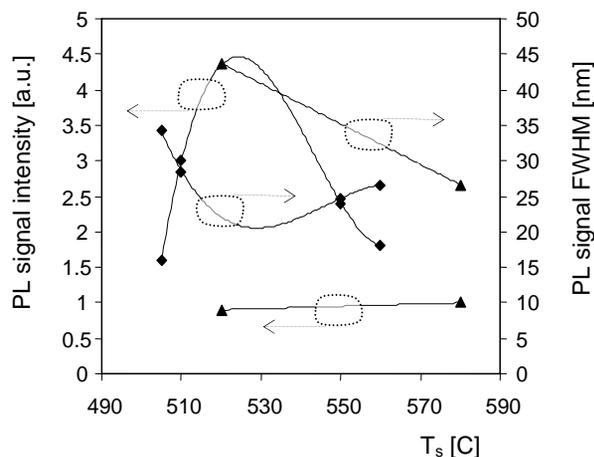
Fig. 2. Room-temperature QW photoluminescence signal intensities (full symbols) and widths (open symbols) for a set of InAlGaAs/AlGaAs/GaAs structures, as a function of crystal surface temperature during growth of quaternary layer. Squares – subseries of epitaxy processes with crystal growth interrupting just before the InAlGaAs deposition, triangles – subseries of runs with temperature ramping (see in the text). Experimental points are connected with the sixth order trend lines.
