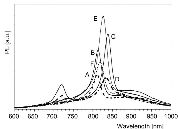
Fig. 1. Room-temperature photoluminescence spectra of a set of InAlGaAs/AlGaAs/GaAs test structures. Letter symbols of structures are placed near the QW peaks.
