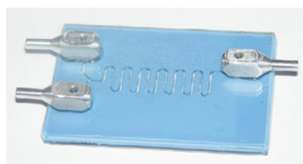
Fig. 5. Real appearance of mixer with microchannels made of LTCC and PMMA layers.
