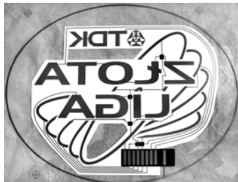
Fig. 2. The view of advertising picture and layers of electroluminescent structure.
