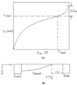
Fig. 1. Definition of  $I_{D_{SAT}}$ ,  $V_{D_{SAT}}$  and  $\Delta I_{kink}$  (a), pinch-off region (b).
