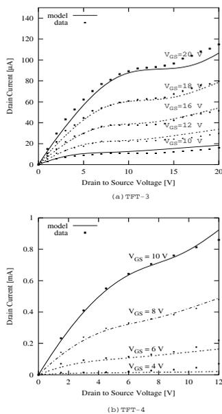
Fig. 3. Output characteristics of TFT3 and TFT4. Curves indicate model results and symbols indicate experimental data.
