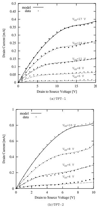
Fig. 2. Output characteristics of TFT1 and TFT2. Curves indicate model results and symbols indicate experimental data.
